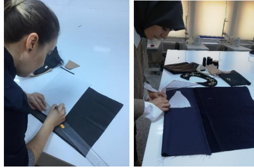
Figure 29-30. Stencil (making a dress pattern) and drawing on fabric by researchers (authors' photograph, 2019).
