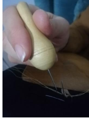
Figure 18. Punching the fabric from the top with us to embroider the upper thread (silvery), ensuring that the lower thread comes out from the pierced point (authors' photograph, 2019).
