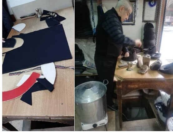
Figure 34. Cutting process of hat pieces (Abdullah Erşan Photography Collection, 2019). Figure 35. Ironing the hat with wooden molds in a steam iron (authors' photograph, 2019).
